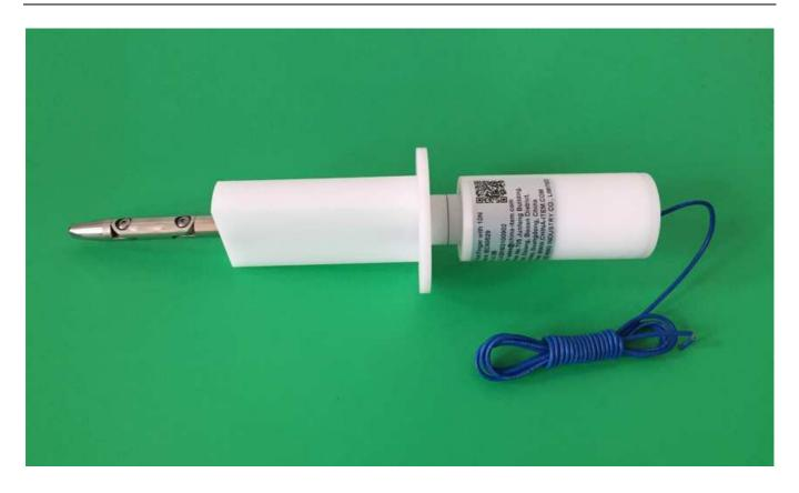
IP2X Test Probe is a precision test probe made according to Figure 1 of the IEC 60529:2013 and is used to simulate a human finger. It is also used by the standards of CSA, IRAM, UL and in most of the rules involved in the verification of accessibility to live parts.
