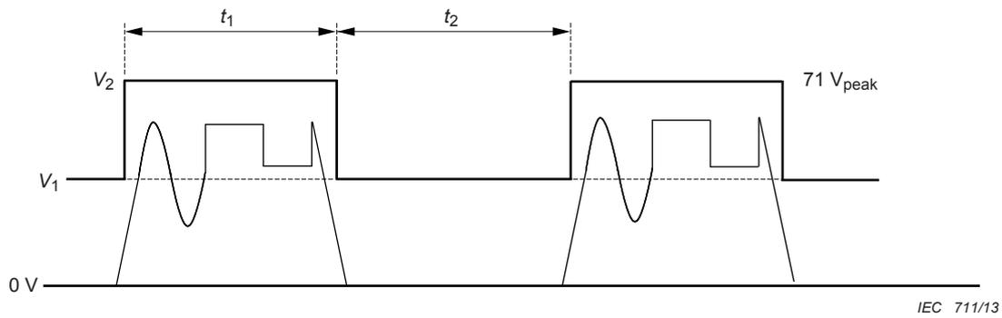
Figure 2E.2 – Voltages in SELV circuits under single fault conditions for multiple pulses above  $V_1$   $\text{A}_2$
