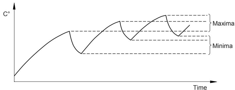
**Figure B.1 – Determination of arithmetic average temperature**
