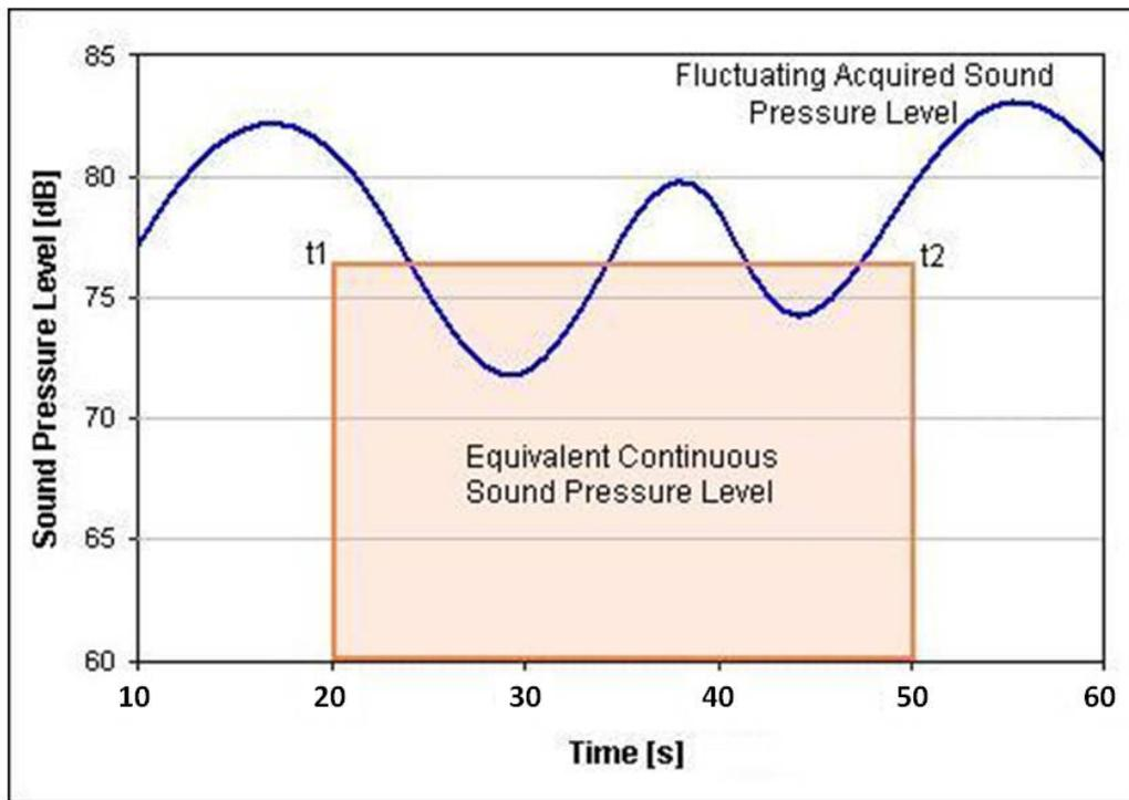
In EN 50332-1 the measurement time interval ( $t_2 - t_1$ ) is 30 s.
