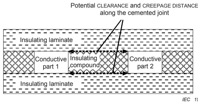
Insulating compound as SUPPLEMENTARY INSULATION or REINFORCED INSULATION
