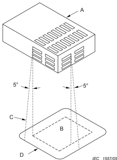
A The portion of a component under which a FIRE ENCLOSURE is required, for example, under those openings in a component or assembly through which flaming particles might be emitted. If the component or assembly does not have its own FIRE ENCLOSURE, the area to be protected is the entire area occupied by the component or assembly.
