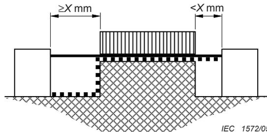
Condition: Path under consideration includes an uncemented joint with a groove on one side less than  $X$  mm wide and a groove on the other equal to or more than  $X$  mm wide.
