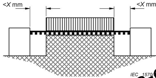
Condition: Path under consideration includes an uncemented joint with grooves less than  $X$  mm wide on either side.
