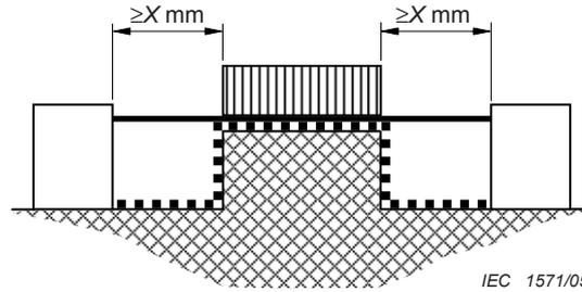
Condition: Path under consideration includes an uncemented joint with a groove equal to or more than  $X$  mm wide each side.
