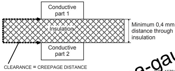
Thick sheet or solid insulating material as SUPPLEMENTARY INSULATION or REINFORCED INSULATION
