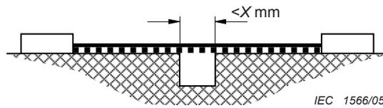
Condition: Path under consideration includes a parallel or converging-sided groove of any depth with width less than  $X$  mm.
