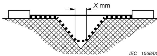
Condition: Path under consideration includes a V-shaped groove with internal angle of less than  $80^\circ$  and a width greater than  $X$  mm.
