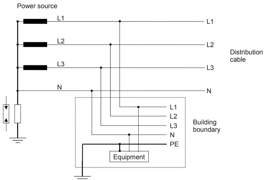
The neutral may be connected to earth through an impedance or surge suppressor, or isolated from earth.
