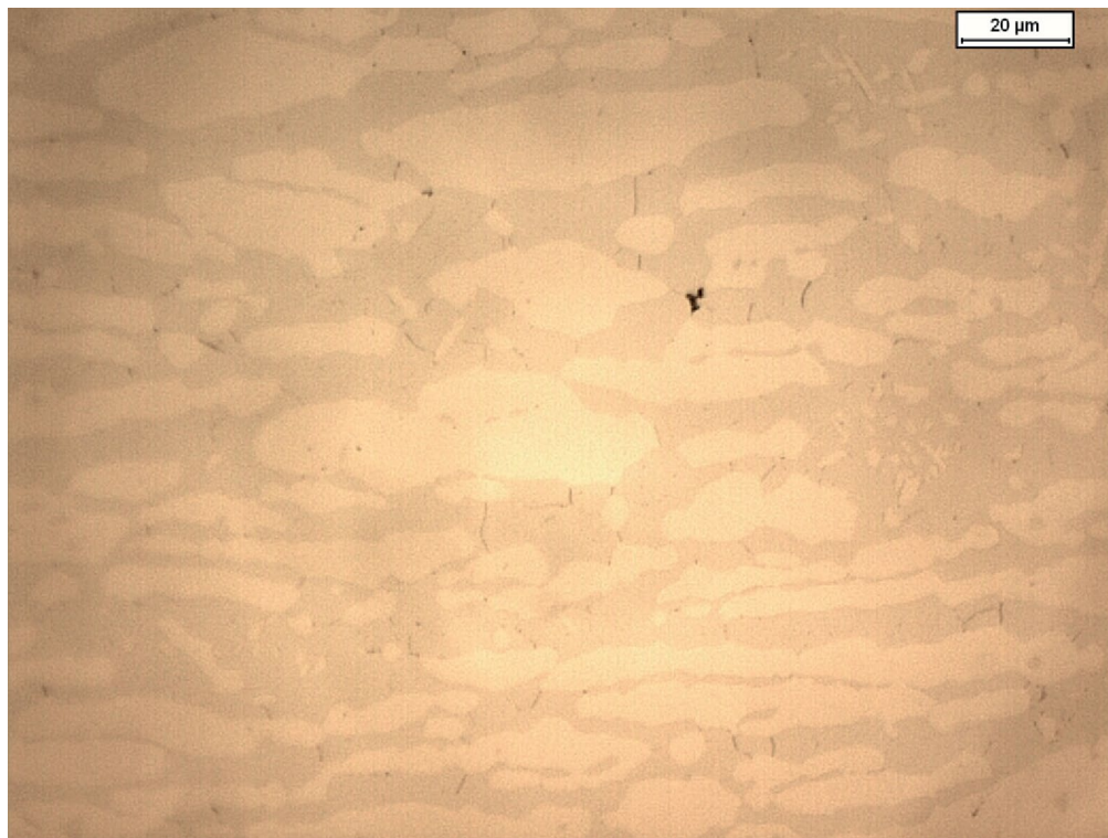
Figure I.1—Just acceptable microstructure: Discrete/standalone intermetallic precipitates not greater than 10 μm (0.40 mil). Electrolytic etching using 10 % NaOH
