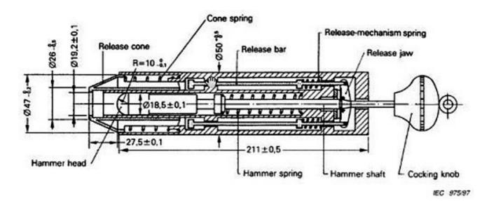
Figure E.1 - Spring hammer test apparatus
