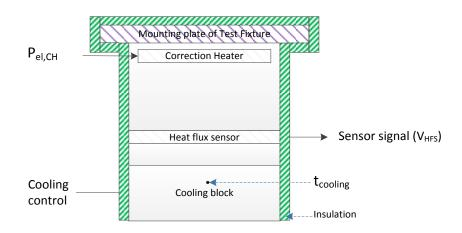
Figure A-2: Calibration of the heat flux measurement setup.
